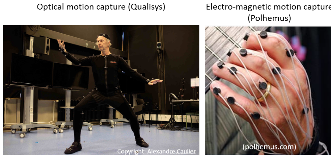
Figure 3.2: State-of-the-art magnetic and optical MoCap systems. Left: Qualisys (optical). Right: Polhemus (electromagnetic).
